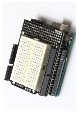
**READ BEFORE INSTALLATION:** Put the component on the side of screen printing and solder on the back of PCB without printing.
